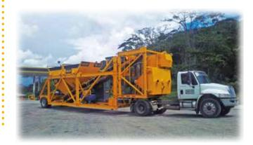
Mobile equipment that dose concrete blends to a mixer truck supplying a high performance in each civil work. To ease work, operation and installation. DP and DT series are compact machines designed to operate in different kind of civil works, minimizing logistic costs. They are planned to be installed in different places to work temporally.
